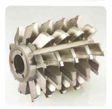
The teeth and body are assembled separately and with different materials.
