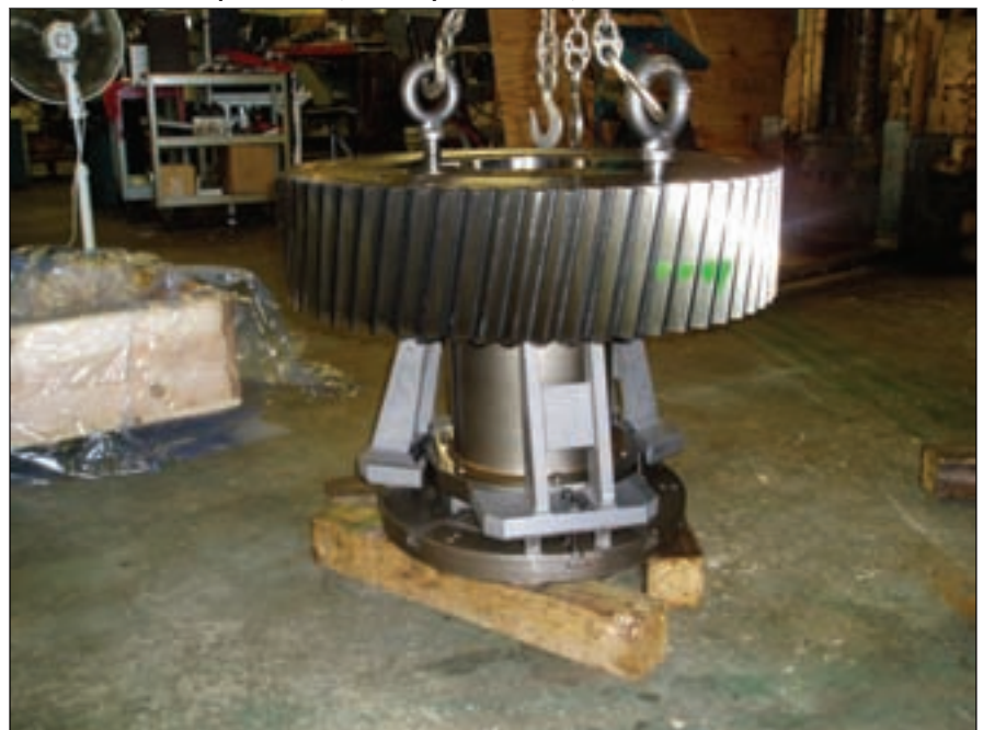
Top: Drewco's workholding system in action. Bottom: The part is held in place by the activation of three pedestals (Courtesy of Rexnord).
